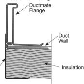
Frequently a contractor installing a high velocity duct system will employ a duct joint with which either he or his work force have no experience. In such a case, it is strongly recommended that the contractor promptly test the initial 100 to 300 feet of duct before installing any more duct. This test will quickly reveal whether or not the workmen can make this joint air-tight in an economical manner.
