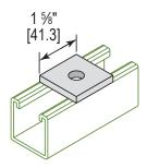
Material is 15/6" [41.3] wide x 1/4" [6.3] thick unless specified. Holes are 3/6" (14.3) diameter, 13/6" [20.6] center to edge on 17/6" [47.6] centers unless specified.
