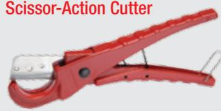
Cut soft plastic tubing and hose quick and easy. Features cast aluminum construction and easy-change, reversible blade for long-lasting performance. Cuts tubing and hose from 1/8" to 1-1/4" (3-31mm) O.D.
