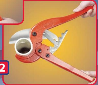
2 Position pipe in the cutter and close handles together to engage ratchet. Blade begins to cut on contact.
