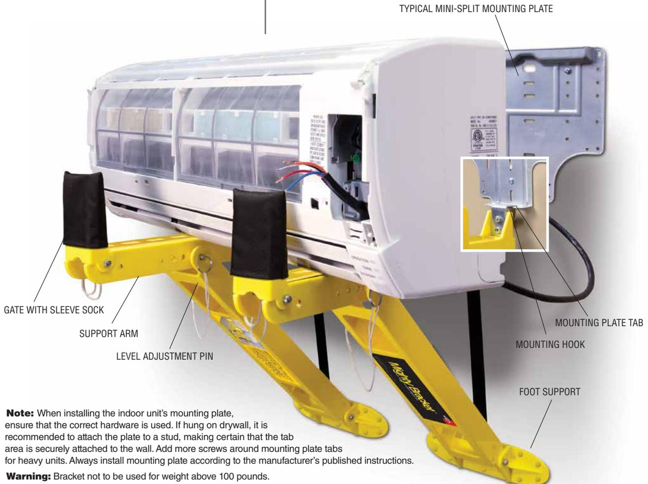
**Note:** When installing the indoor unit's mounting plate, ensure that the correct hardware is used. If hung on drywall, it is recommended to attach the plate to a stud, making certain that the tab area is securely attached to the wall. Add more screws around mounting plate tabs for heavy units. Always install mounting plate according to the manufacturer's published instructions.
