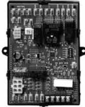
**Universal electronic fan control for gas furnaces, replaces multiple Honeywell models. Includes instructions and special wire harnesses for easy replacement.**
