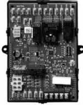
**ST9103A integrates control of burner and circulating fan operations in an oil furnace. Two speed circulator for oil appliances. Isolated line voltage limit interface and isolated relay connection to oil primary.**
