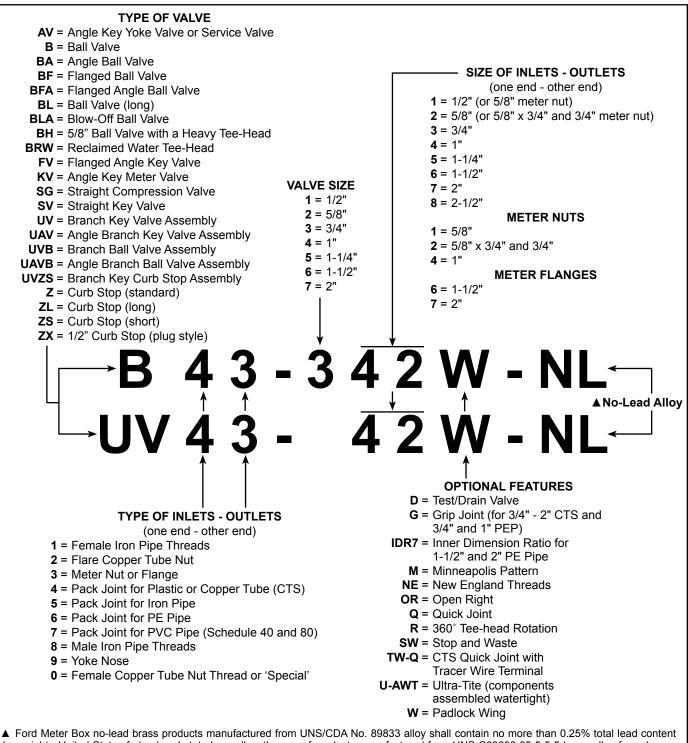
A Ford Meter Box no-lead brass products manufactured from UNS/CDA No. 89833 alloy shall contain no more than 0.25% total lead content by weight. United States federal and state laws allow the use of products manufactured from UNS C83600 85-5-5-5 brass alloy for only non-potable water systems within the United States. The same UNS C83600 85-5-5-5 brass alloy, also referenced as gunmetal or LG2, is specified and used in potable water systems in most other countries.
