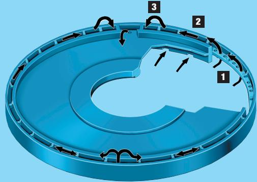
**HOW THE ZURN DIAPHRAGM WORKS**
