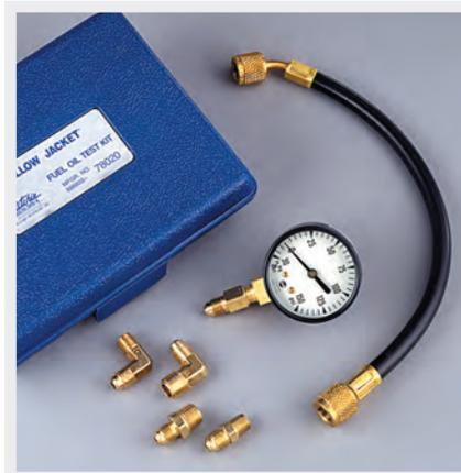
Determine pump efficiency, cut-off and suction, as well as analyze or troubleshoot burner efficiency. Kit includes 2" gauge, 30" 0-150 lb. scale and 12" hose with fittings.
