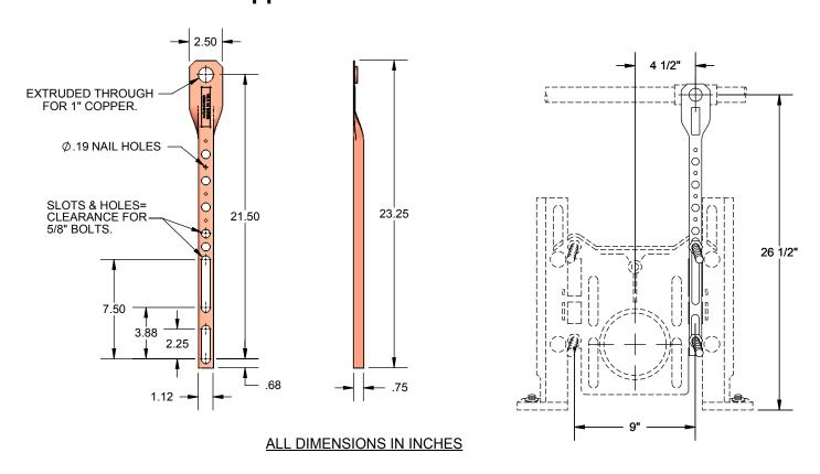
The HOLDRITE #114-C is a Copper-Bonded™ steel bracket with two slots for securely mounting upright to the carrier unit. The top end has a single 1-1/8" extruded hole for soldering 1" copper pipe, as well as supporting the water pipe for the flush valve above the floor. Adjust the flush valve 4-1/2" from the carrier center and 14" above the top fixture mounting bolt. This installation typically places the flush valve at 11-1/2" above the fixture, When soldering, heat the pipe, not the bracket.
