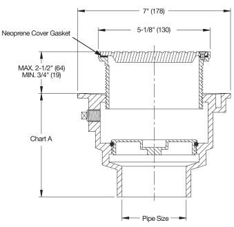
Load Rating \*XHD \*The load classifications are in accordance with the American National Standards ASME A112.21.1M ASME Ratings are as follows:
