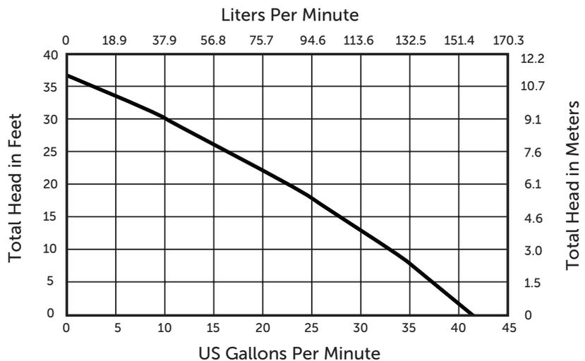
**Note:** Maximum shut-off head is 36'. Usable maximum head - assuming 150' of lateral discharge through 1" pipe is 25'. Consult factory for proper sizing and calculation of friction loss.
