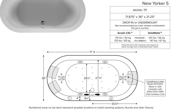
When Fill-Flush is ordered and location 2 is chosen, the detergent feeder will need to be offset to the left or the right. Shown with Air Massage and Ultra Whirlpool Package.
