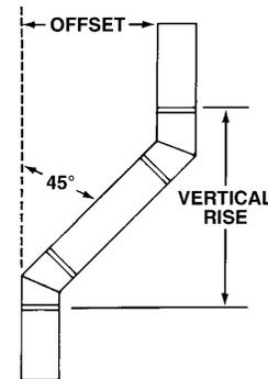
Note: The vertical rise can also be closely estimated by adding one "A" and one "B" dimension to Maximum Offset figures. (See dimensions of Round Adjustable 45° Elbows.)
