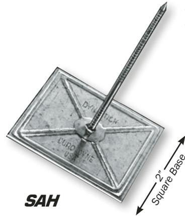
SAH Dynastick is an insulation hanger with a self-stick base. Just peel the release paper from the hanger base and firmly press the base to the clean duct surface. Impale the insulation over the hanger nail and slip on the locking washer. Self-stick hangers adhere to clean metal surfaces and withstand temperatures of up to 175 °F.
