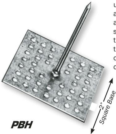
PBH Dynastick is a perforated base hanger for use with super strength PBA mastic. Simply place a small amount of PBA on a perforated base and firmly press the hanger against the duct surface. Allow the PBA mastic to dry, then, impale the insulation over the hanger nail and slip on the locking washer. Duro Dyne PBA adheres to concrete, metal or wood surfaces and withstands constant temperatures up to 180 °F.
