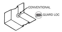
All Duro Dyne Flexible Duct Connector Products are suitable for pressures of -10 to +15 wg. Duro Dyne's standard 'single fold' metal to fabric grip has been tested by an independent testing laboratory to withstand a negative pressure of -10"WC and a positive pressure of +17.25" WC with no tearing or visible separation.
