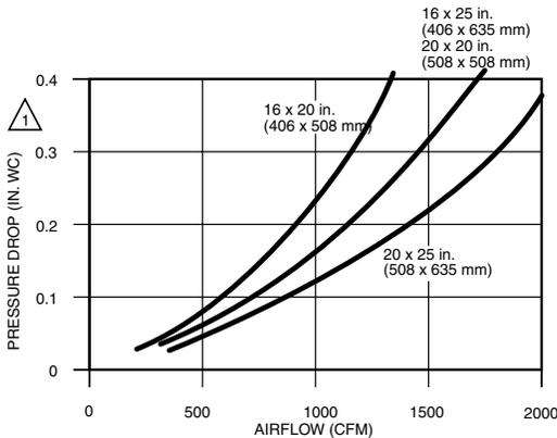
⚠ WHEN FIRST INSTALLED, PRESSURE DROP INCREASES AS FILTER BECOMES LOADED. REPLACE FILTER WHEN PRESSURE DROP REACHES 0.5 IN. WC. (0.1 kPa).
