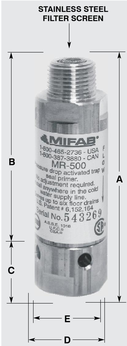
**Specification:** MIFAB® model MR-500-NPB pressure drop activated brass trap seal primer, with inlet opening of ½" (13) male N.P.T. and outlet opening of female ½" (13) N.P.T. Complete with four view holes and removable filter screen. Serves up to 6 floor drain traps and requires no adjustments and no air pre-charge.
