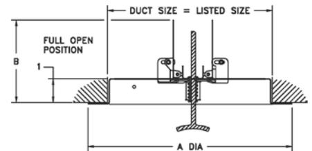
**Note:** Knob permits diffuser to be held in position while attaching face screws.
