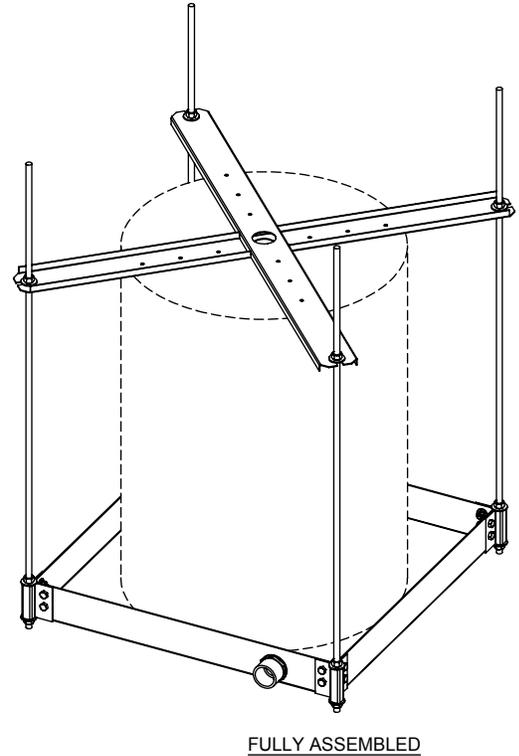
The Suspended Water Heater Platform is engineered to support water heaters up to 20 U.S. gallons (up to 375 pounds total weight). This time and labor savings tool is designed for the Professional Contractor. Design features requested by plumbers are incorporated into a professional platform that can be suspended with all thread rod.
