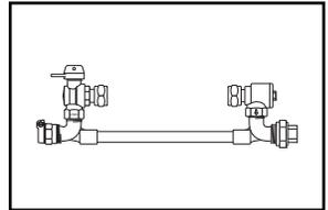
**ANGLE BALL VALVE BY ANGLE DUAL CHECK VALVE**
