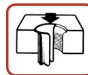
**FORMS STRONGER FLARES**- Stronger flares assured by smooth, even radius formed at base of every flare by engineered chamfer.
