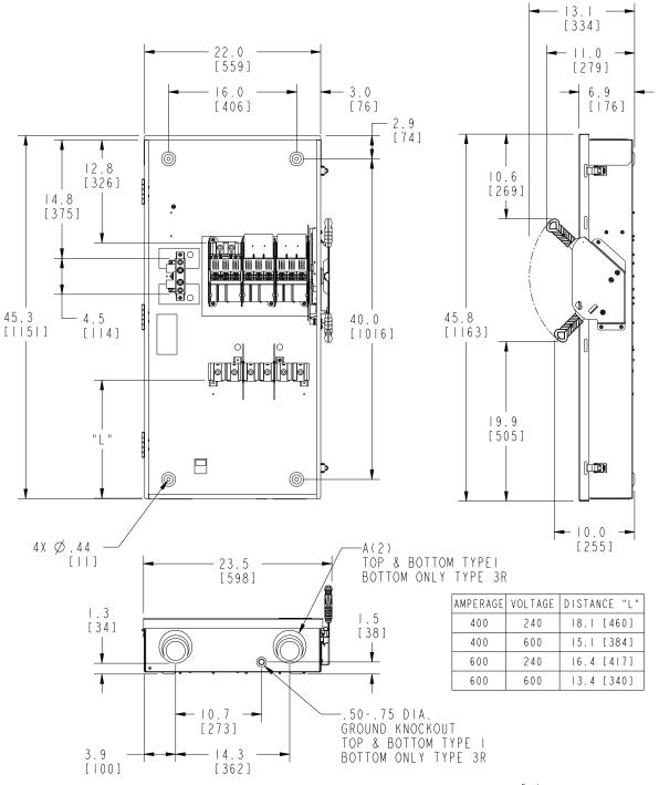
Dimensions shown in inches and millimeters [ ]. Dimensions shown accurate to  $\pm$  1/8 inch.
