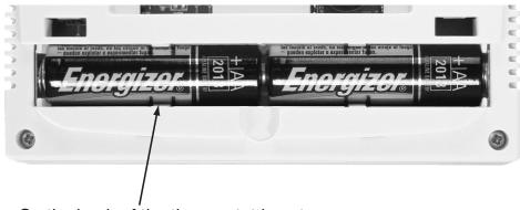
On the back of the thermostat insert 2 AA Alkaline batteries (included).
