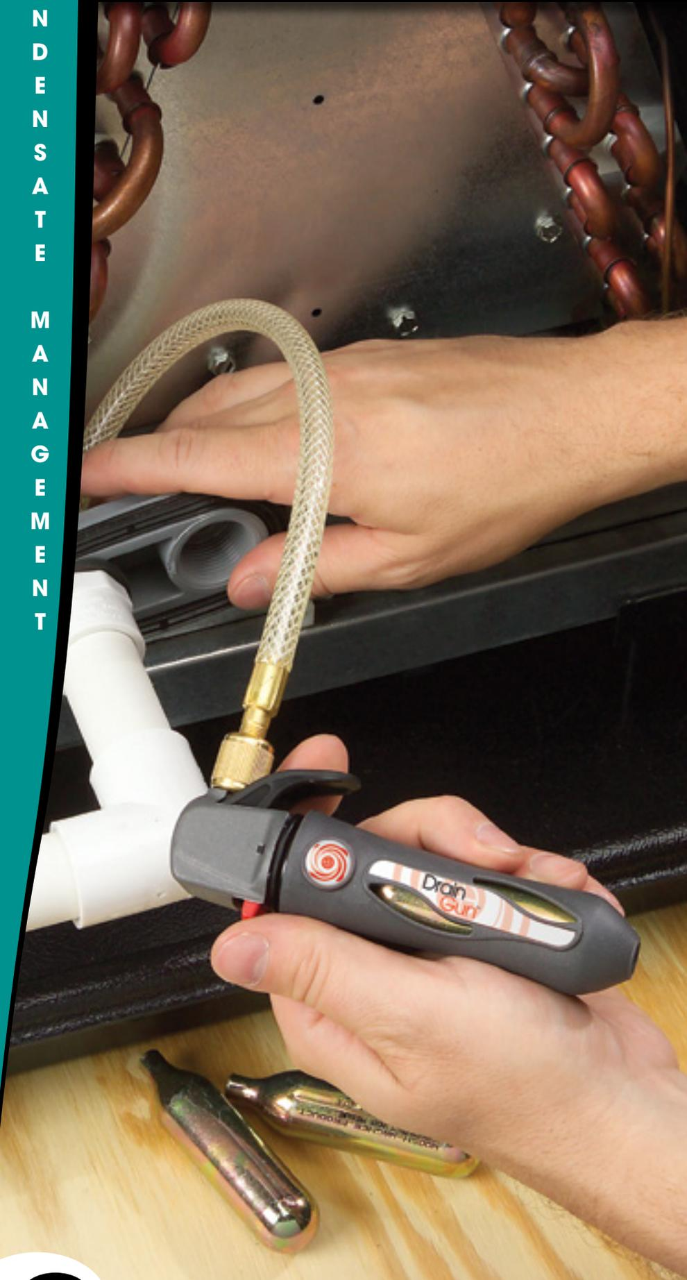
**T**he Drain Gun - Charles Gallo Brand is a lightweight (3oz.) portable tool designed to blow out condensate drain lines instantly. Simply insert a Swoosh CO<sub>2</sub> cartridge into the Charles Gallo Drain Gun and with a press of the trigger — SWOOSH — 800 psi of oil free air clears the line.
