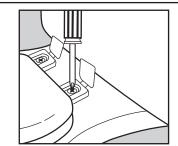
Tighten the bolts using your screwdriver.
