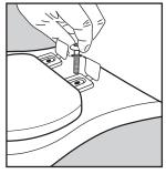
When the seat is properly aligned with the front edge of the bowl, slip the bolt through the washer and the bowl bolt holes.
