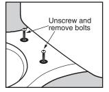
Once plug is in place, unscrew and remove bolts and keep nearby for step 4.
