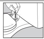
When the seat is properly aligned with the front edge of the bowl slip the bolt through the bowl bolt holes.
