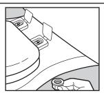
With the plastic bolts installed, thread the winged plastic nuts on to the bolts.
