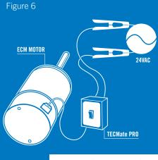
NOTE: The high voltage 5-Pin connector must be connected to the motor for TECMate tests.
