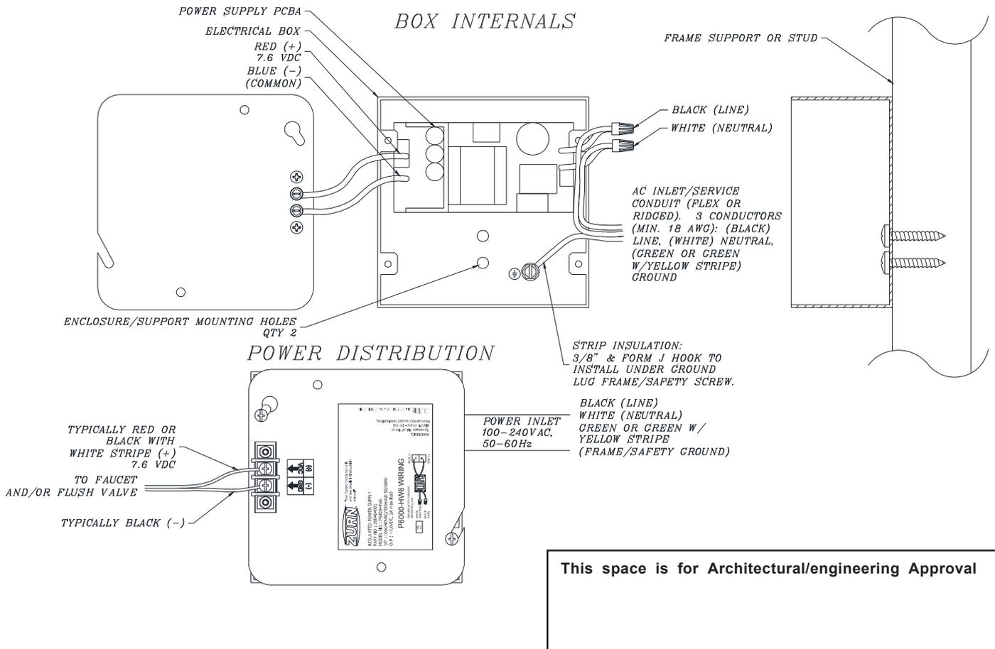
**ENGINEERING SPECIFICATION: ZURN P6000-HW6 Power Converter** - The Hardwired Power Converter is a 7.6 VDC regulated, 2.0A power supply that will operate up to: (8) ZEMS or ZEMS-IS Sensors/Actuators, (8) ZESS Sensors/Solenoids, (8) sensor faucets, or (8) Pint Urinal valves. The unit shown above is integrated into a 4"L x 4"W x 2-1/8"D electrical box. The AC input connections are terminated within the electrical box. The 7.6 VDC output terminals are externally mounted to the cover plate.
