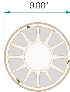
Constructed of 2 circular bands with 3 braces.
