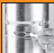
To unlock, simply bend out the tab.
