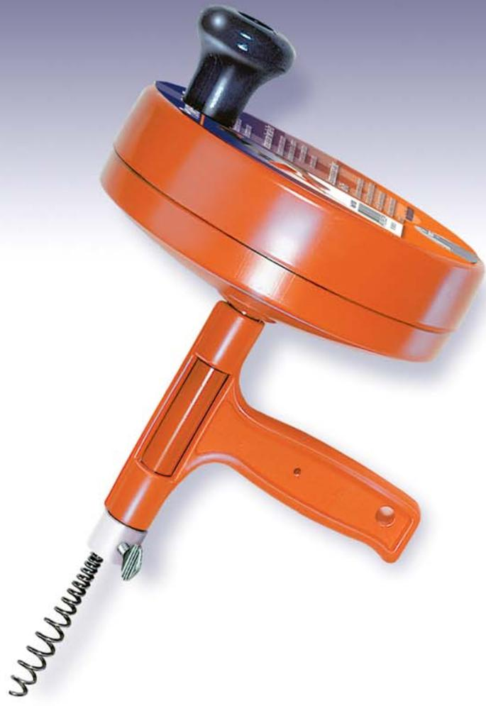
**S**urprising quality in a low-priced tool. Cable is held in place with a thumb screw. Stamped steel drum has a 25 ft. capacity. High impact "T" handle is particularly convenient for use in laundry tubs. Cables are economy grade for light duty occasional use.
