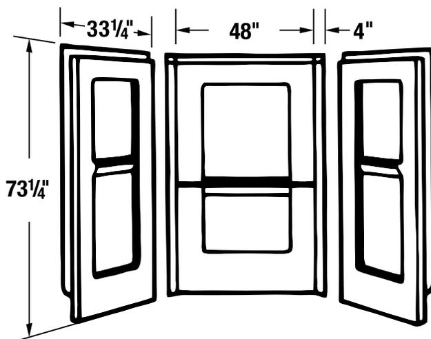
**General:** Furnish and install as shown on plans, 32" x 48" rectangular shower, DURAWALL® Shower Walls Model 748-34, as manufactured by E.L. Mustee & Sons, Inc. Shall be 3-piece, molded fiberglass wall with minimum thickness of 125 mils and mounts direct-to-studwalls. Includes center panel with molded-in shelves and two side panels with molded-in shelf. Self aligning panels use a tongue-and-groove connection. Shall meet ANSI Z 124-2011.2. Color \_\_\_\_ (White, Bone).
