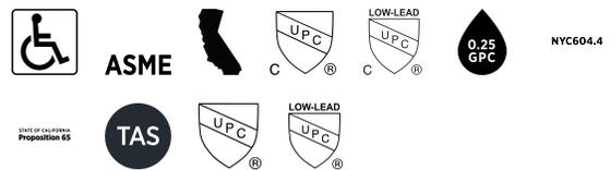
(ADA Compliant, ASME A112.18.1 Compliant, CEC Compliant, cUPC Certified, cUPC Low Lead Compliant, GPC 0.25 or less, NYC604.4, Proposition 65, TAS, UPC Certified, UPC Low Lead Compliant)
